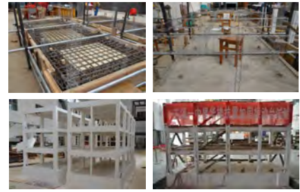
The reinforced concrete frame structure, strengthened with buckling-resistance braces, underwent a shaking table test.
