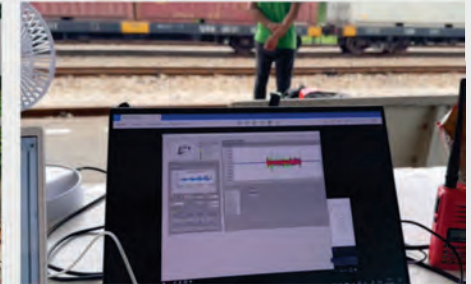
The TWD are measuring weight of the train.
