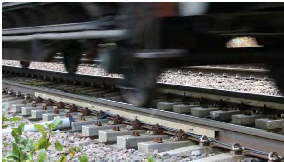
Example photograph: The Tamtron Scalex Wild wheel impact measuring system
