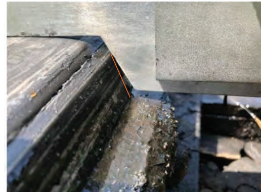
Gauge No.4, Switch No. 214, 20 in from the tongue's end Test at Bangsue Locomotive Depot
