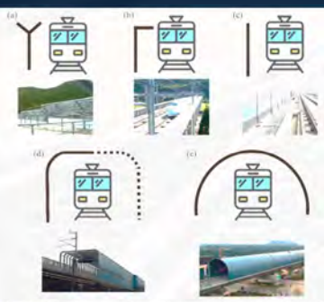
Figure 6. (a) Undeveloped sound barrier; (b) inverted L-shaped sound barrier; (c) upright top-sound barrier; (d) wall-enclosed sound barrier; (e) fully enclosed sound barrier. Ref: Yan, Hongyu, et al. "A review of recent research into the causes and control of noise during high-speed train movement." Applied Sciences 12.15 (2022): 7508.
