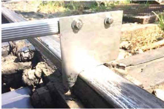
Gauge No.1, Switch No. 214, 5 in from the tongue's end Test at Bangsue Locomotive Depot
