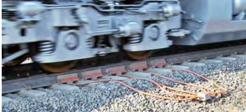
Example photograph of WILD system installed on the way-side of track.
