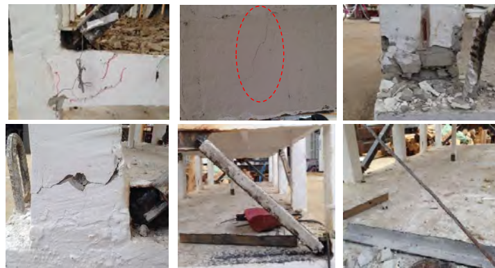
The reinforced concrete frame structure, strengthened with buckling-resistance braces, underwent a shaking table test.
