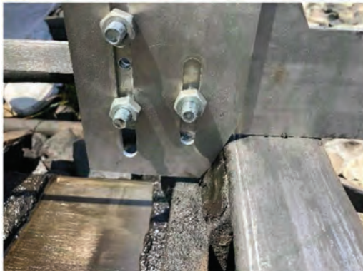
Gauge No.3, Switch No. 214, 2 in from the tongue's end Test at Bangsue Locomotive Depot
